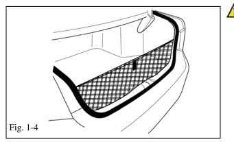
(e) Confirm completed assembly. Make sure net handle is facing out toward the rear of the vehicle (Fig. 1-4).
